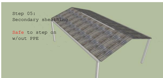
Figure 10. While modeling in a BIM application does not provide enough information about the safety during the construction process, embedding layer information in the panel's object family will determine when the panel is safe.
